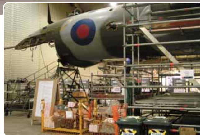
The most famous Avro Vulcan in the world sits inside the VTST hangar during May 2006, completely stripped down and in the middle of its major overhaul.
