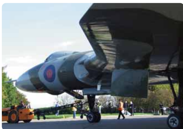
The cranked-delta wing of the Vulcan is clearly evident in this shot – the modification was made to the wing very early on in the aircraft's history, although early test airframes did fly with straight leading edges.
