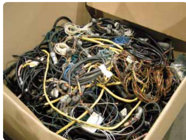
Many miles of cabling have been removed from the now civil-registered G-VLCN, mostly relating to the now redundant military systems.
