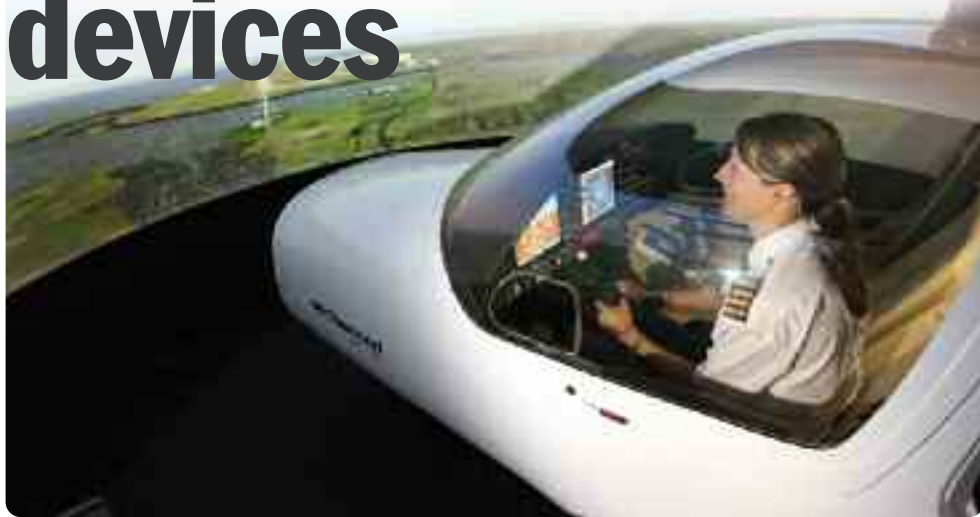
One of CTC's four new DA42 simulators, with enhanced CAE TROPOS visual system
