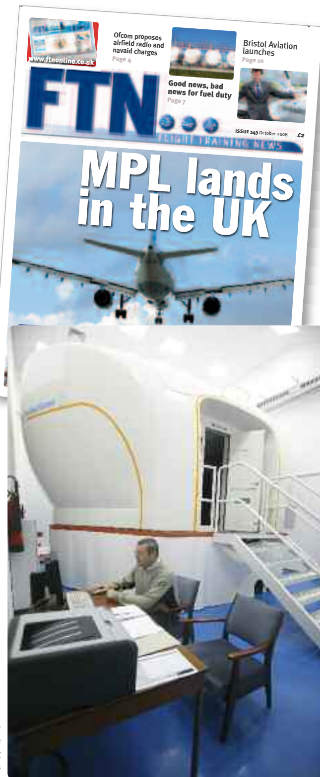
The MPL's key training device based at FTE, a Mechtronix FFT-X Boeing 737NG FSTD
