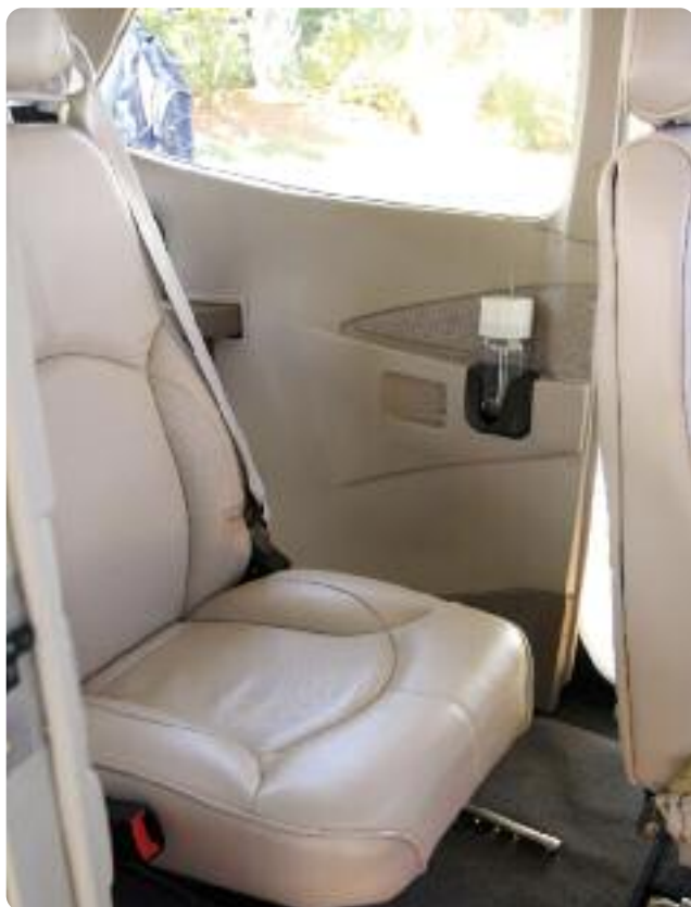
The new single rear seat configuration designed for flight school operation
