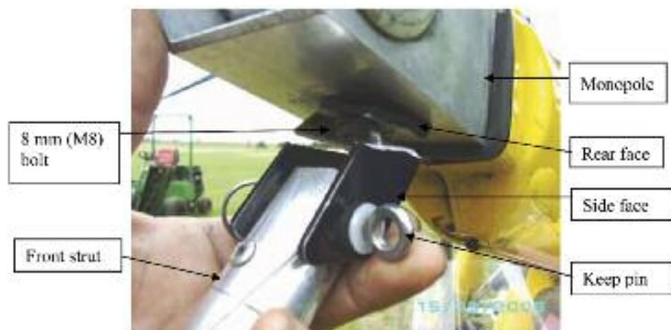
Figure 1 - Failed front strut bracket
